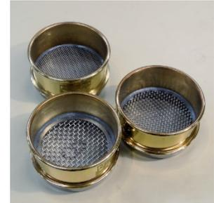
Figure 8. Calibrated Sieves
